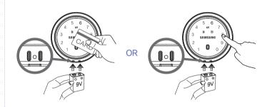
While contacting a 9V battery to the external power (emergency battery) contact on the outer body for 2 seconds or longer, place the card or key tag or enter the password
