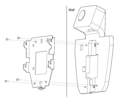
4 Install FaceStation 2 onto the fixed bracket.
