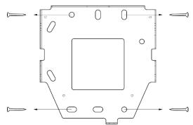
**3** Fix the thermal camera module bracket firmly using fixing screws to the position where FaceStation 2 will be installed.
