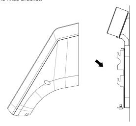
**6** Connect FaceStation 2 to the bracket by rotating the product fixing screw of FaceStation 2.
