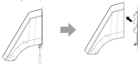
**2** Loosen the fixing screws to separate the bracket from the wall.
