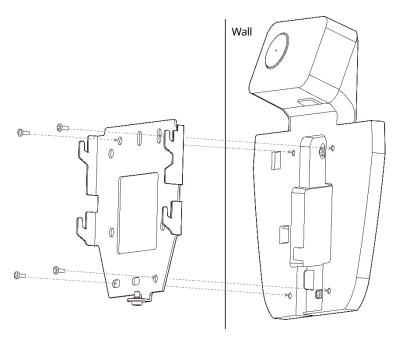
5 Install FaceStation 2 onto the fixed bracket.
