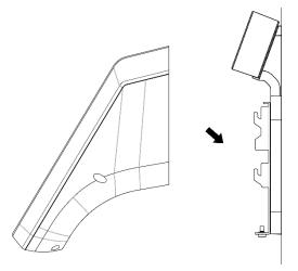
**5** Connect FaceStation 2 to the bracket by rotating the product fixing screw of FaceStation 2.
