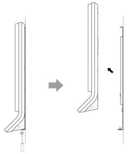
**2** Loosen the fixing screws to separate the bracket from the wall.
