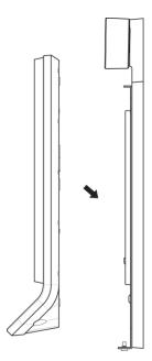
**6** Connect FaceStation F2 to the bracket by rotating the product fixing screw of FaceStation F2.
