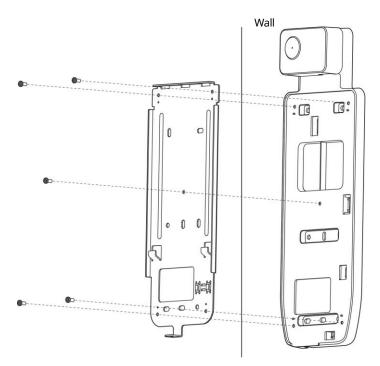
4 Install FaceStation F2 onto the fixed bracket.
