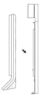
**5** Connect FaceStation F2 to the bracket by rotating the product fixing screw of FaceStation F2.
