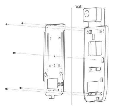
**5** Install FaceStation F2 onto the fixed bracket.
