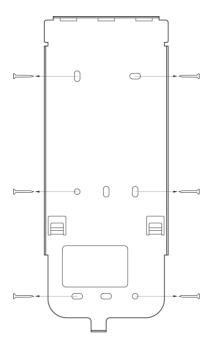
**3** Fix the thermal camera module bracket firmly using fixing screws to the position where FaceStation F2 will be installed.
